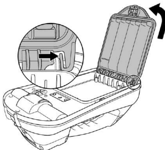
Figure 4.5: Press the release catch and lift the battery pack away
