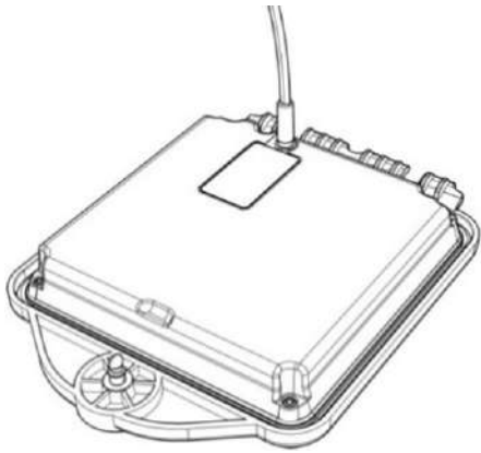
Figure 4.8 Charging the transmitter Li-Ion battery pack
