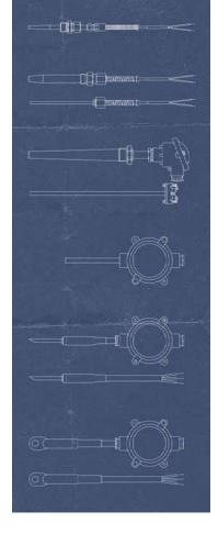
**Temperature** Sensors are ideal for maritime applications including, but not limited to: measuring exhaust gases and cooling water in diesel engines, product temperatures, and room temperatures in refrigeration stores. The temperature sensors are designed with high resistance against vibration.
