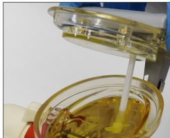
***Baffle plate must come in contact with the oil***
