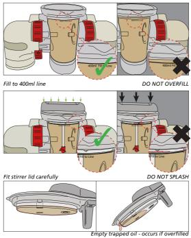
Figure 4 Filling the test vessel
