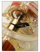
Setting the electrode gap accurately is very important; the results obtained are only valid if the gap is correct. A big problem is movement of the electrodes after the gap has been set and for this reason, many users of oil test sets check the electrode gap frequently – sometimes before every test. A better solution is to use test sets where the electrodes can be locked in position, such as the instruments in Megger's latest OTS range.
