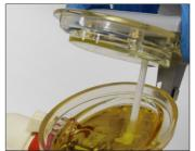
Baffle plate must come in contact with the oil Figure 3
