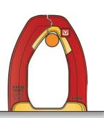
The display shows (a) to indicate that the measurement is from the jaw. When the current measurement is < 0.5 A, the center dot in the icon flashes. For current measurements > 0.5 A, the center dot in the icon is steady.
