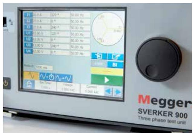
Stand-alone functionality in the field. With its built-in LCD touch-screen and USB port, SVERKER900 needs no PC.
