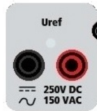
Figure 7 AC/DC AUX V4 Output Terminals
