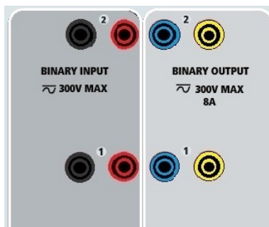
Figure 5 Binary Inputs and Outputs 1 and 2
