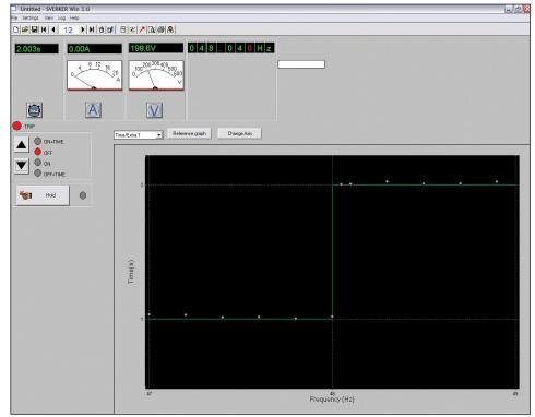
Testing frequency relay with SVERKER 780
