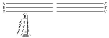
First, it will indicate the presence of a voltage on the touched line, by means of a flashing light and beeping sound.
