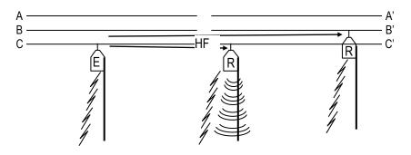
The transmitter and the receiver include an integrated tests system by which all the modules are tested: electrical components, battery, wiring and antenna. Carrying out the test corresponds to a real line touch.
