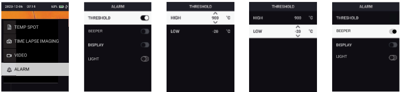
Figure 11.16 Configuring the high and low alarms.
