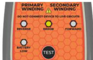
Figure 1.5 Amber LED 1 second flash
