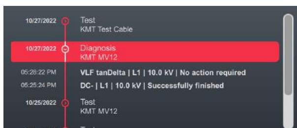
This makes all measurement data records contained in this directory and the associated metadata (time, operating mode, phase, voltage and comment by tester) visible.
