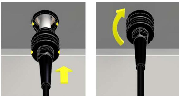
3. Connect the other end of the HV cable to the test object.
