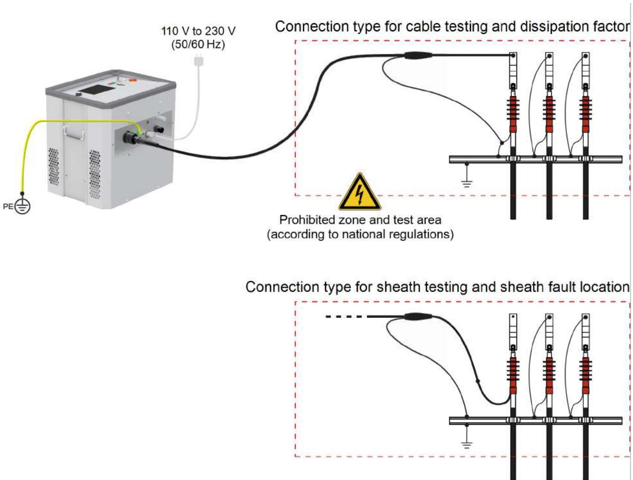
To connect the test system to the test object, proceed as follows:
