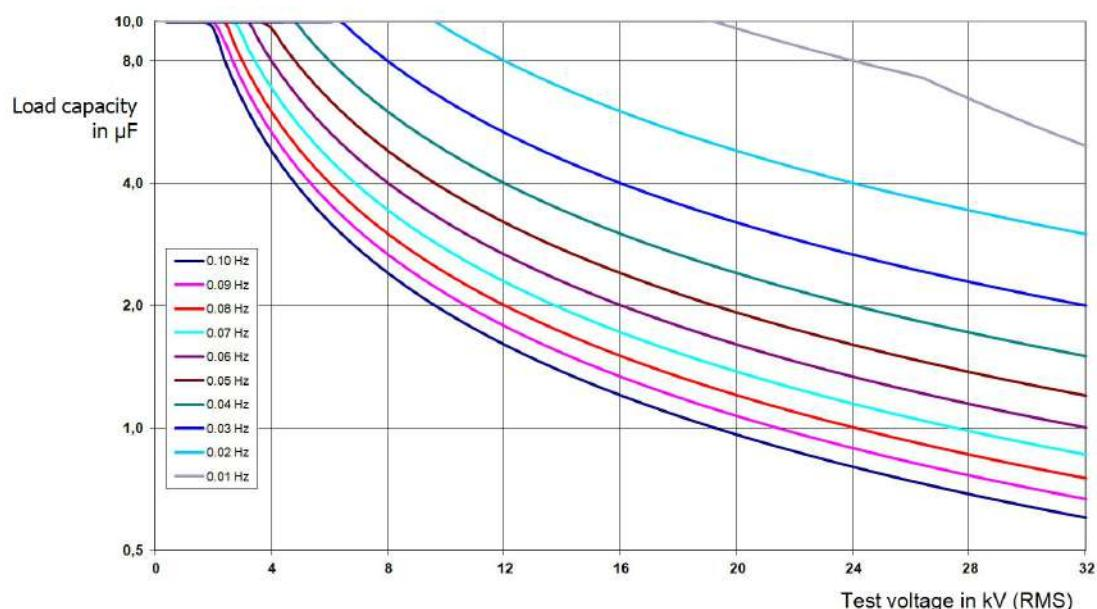
For **cosine rectangular voltage and damped AC voltage (DAC)** (boost module required), the following load diagram applies as and where appropriate<sup>1</sup>:
