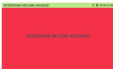
At the same time, internal earthing of the HV output is prevented to protect the operator and the system.
