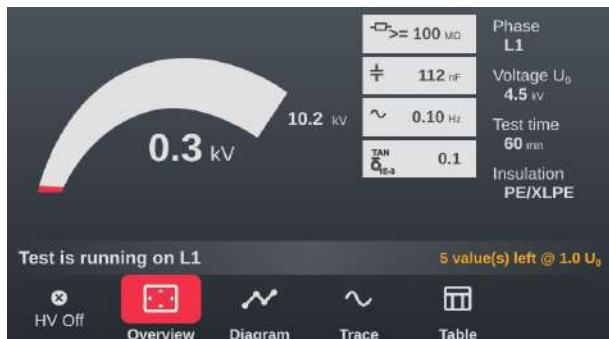
In addition to the current test voltage and the remaining test duration (or the remaining measured values in the step test), this also displays the following measured values:
