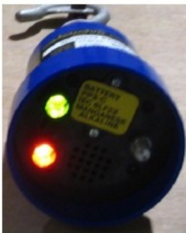
WPC2000 Receiver showing Line Live In-Phase Condition with Transmitter
