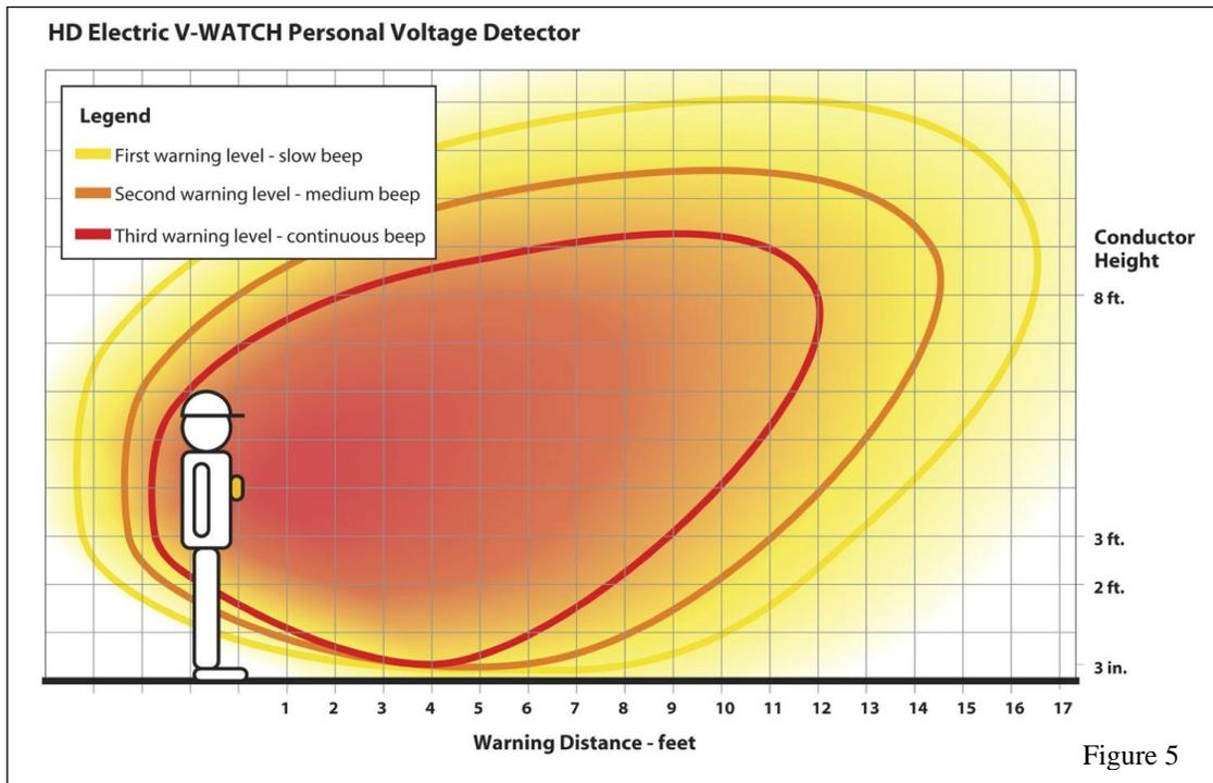
The presence of live conductors in the zone of optimum sensitivity will provide an audible and visual warning to the user from a distance of 2 to 5 meters (6.5 to 16 feet).
