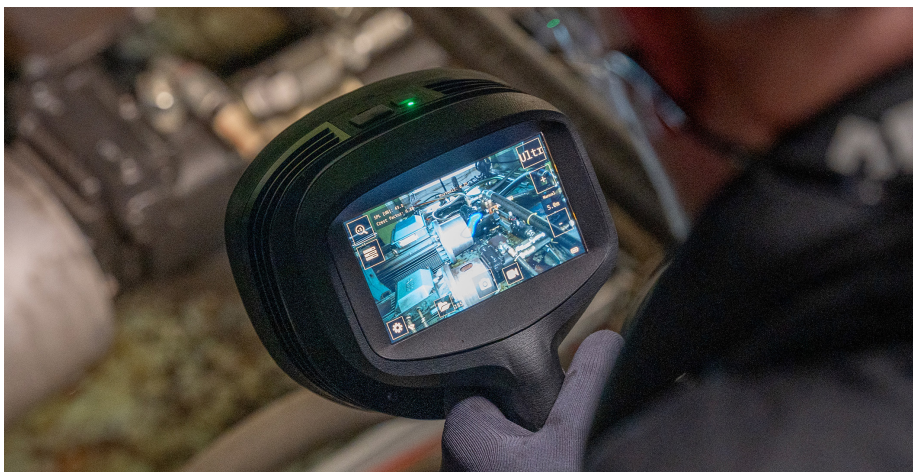
The Flir Si2-Pro helps prevent failures by detecting mechanical issues at an early stage in critical components of equipment, such as gearboxes, conveyors, and other rotating machinery.
