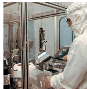
Deposition of photosensitive resin during studies of optical chips.
