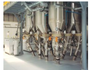
The new CCM™ (Continuous Compound Mixing) technology, integrated into a MIRS™ plant at Bicocca, Milan.
