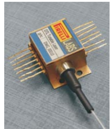
Widely tunable laser, for optical networks, produced in the Pirelli Labs.
