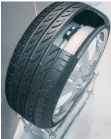
The X-Pressure System™ for measuring the air pressure inside the tyre.
