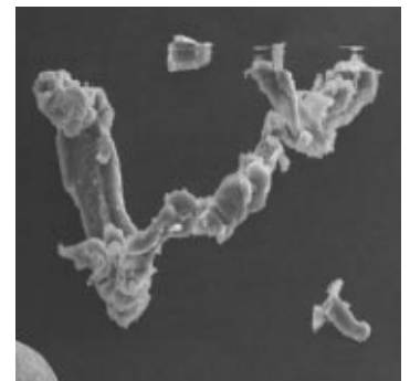
Real tyre debris particles at scanning electron microscope (dimension of the largest particle around 0.3 mm)
