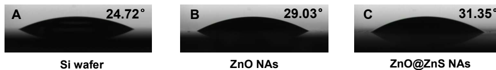
Figure S14. Photographs of water contact angle measurements on the surfaces of: (A) Si substrate, (B) ZnO nanorod array, and (C) ZnO@ZnS nanorod array. The results showed that the obtained array substrates are highly hydrophilic.
