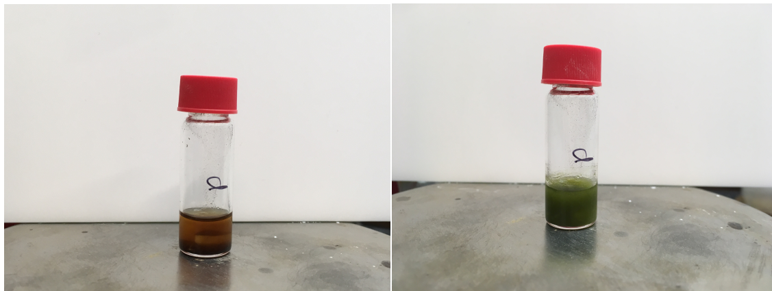
Figure S1. Preactivation of the catalyst. Left: before preactivation, showing red color from catalyst 3 . Right: after preactivation, showing green color of the Ti III active catalyst.
