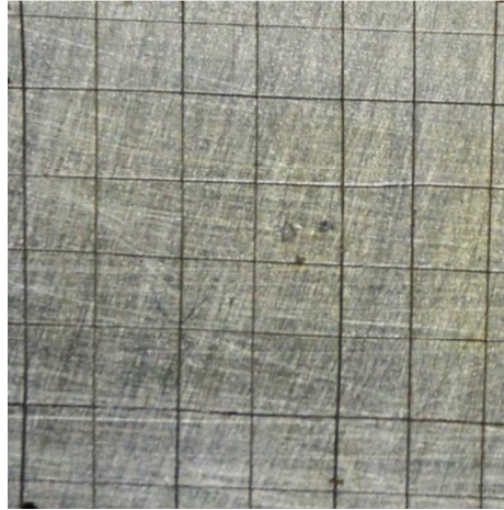
Figure S5 The digital photo of the sample after taping test according ASTM D3359-17 (test method B).
