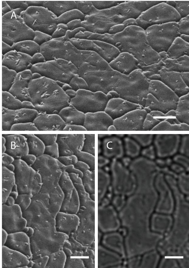
Figure S2: (a) Raw SEM image. (b) Rotated and scale-corrected SEM image. (c) Optical microscopy image. All scale bars are  $3 \mu\text{m}$ .
