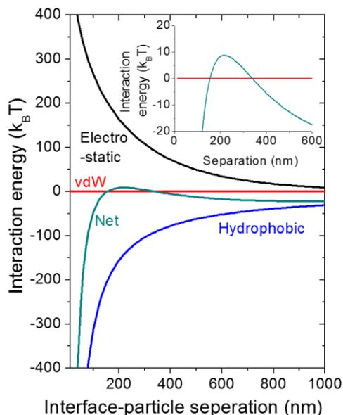
**Fig. S4.** Pair interaction energy between a lignin NP and a flat oil-water interface as a function of interface-particle distance. The net interaction energy is the sum of electrostatic, van der Waals and hydrophobic interactions between the lignin NPs and decane-water interface.
