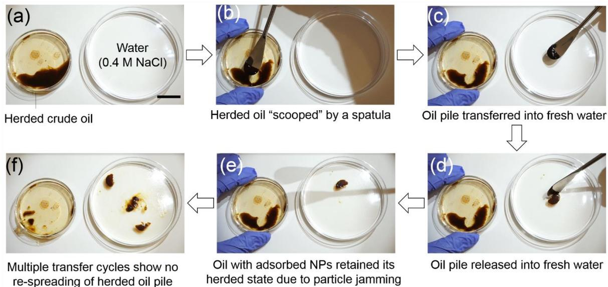
**Fig. S9.** (a-f) Sequence of images showing the transfer of herded oil slick into fresh water surface contained in a Petri dish. The crude oil herded with lignin NPs-pentanol mixture retained its herded state on the fresh water surface. This ability to retain droplet shape highlights that the lignin NPs are irreversibly adsorbed on to the interface, which further restrict re-spreading of the oil onto water surface. Scale bar shown in (a) is 2 cm.
