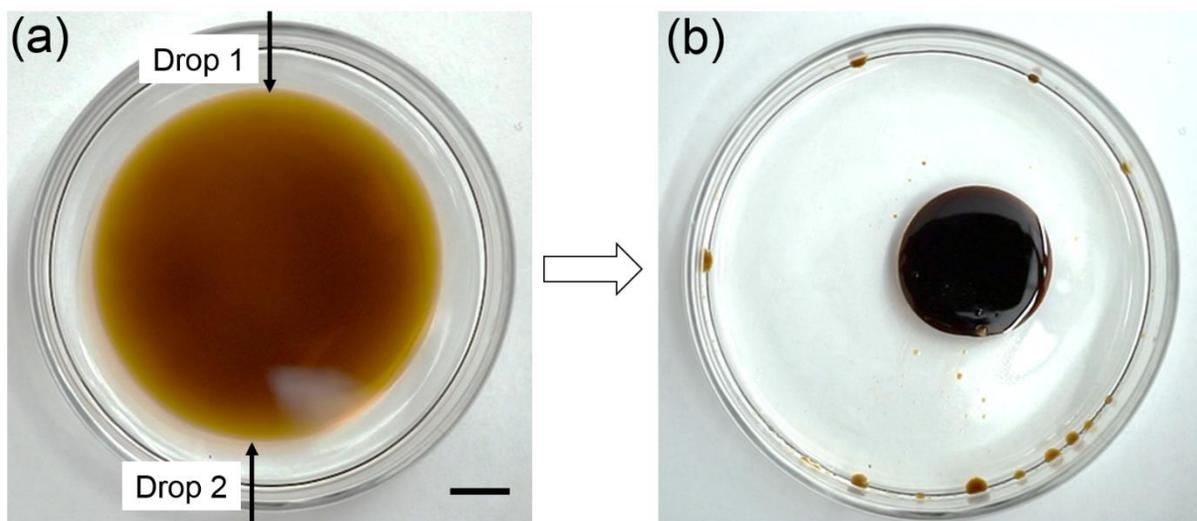
**Fig. S8.** (a-b) Images showing herding process by adding two droplets of lignin NPs-pentanol mixture from direction indicated by the arrows in (a). The herded oil slick is at the center of petri dish due to the Marangoni flow and interfacial mass transfer generated by two droplets. Scale bar shown in (a) is 1 cm.
