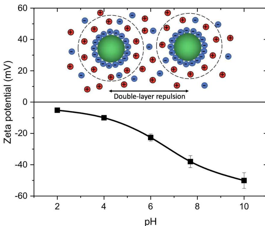
**Fig. S2.** Zeta potential of lignin NPs as a function of pH. The isoelectric point of the particles is  $\text{pH} < 2$ , and particle dispersion remains stable at wide range of pH (4-10) due to electrostatic repulsion. The inset schematic shows the principle of double layer repulsions, where the overlap of the diffused counter ion layer induces a repulsive osmotic pressure that stabilizes the particles.
