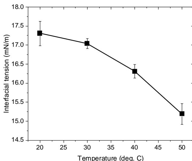
**Fig. S5.** Interfacial tension between crude oil and 0.1 mg/ml lignin NPs dispersion containing 0.4 M NaCl solution. The interfacial tension decreases with increasing temperature. This is attributed to faster diffusion of NPs toward the oil-water interface at higher temperatures.
