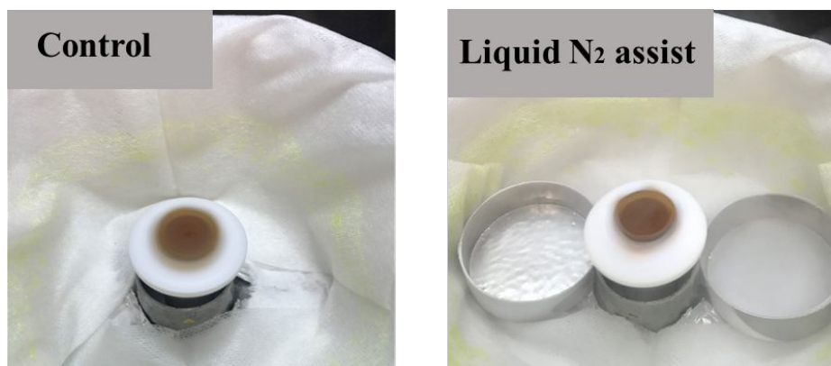
Fig. S3 One-step anti-solvent method for preparing perovskite films. (a) Conventional process and (b) liquid nitrogen assist process, the ambient temperature is about 23 °C and the temperature during spin-coating was about 4 °C.
