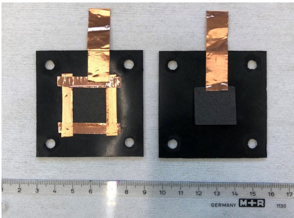
**Fig. S3:** Sealing of the conducting tape to the gas-diffusion layer.
