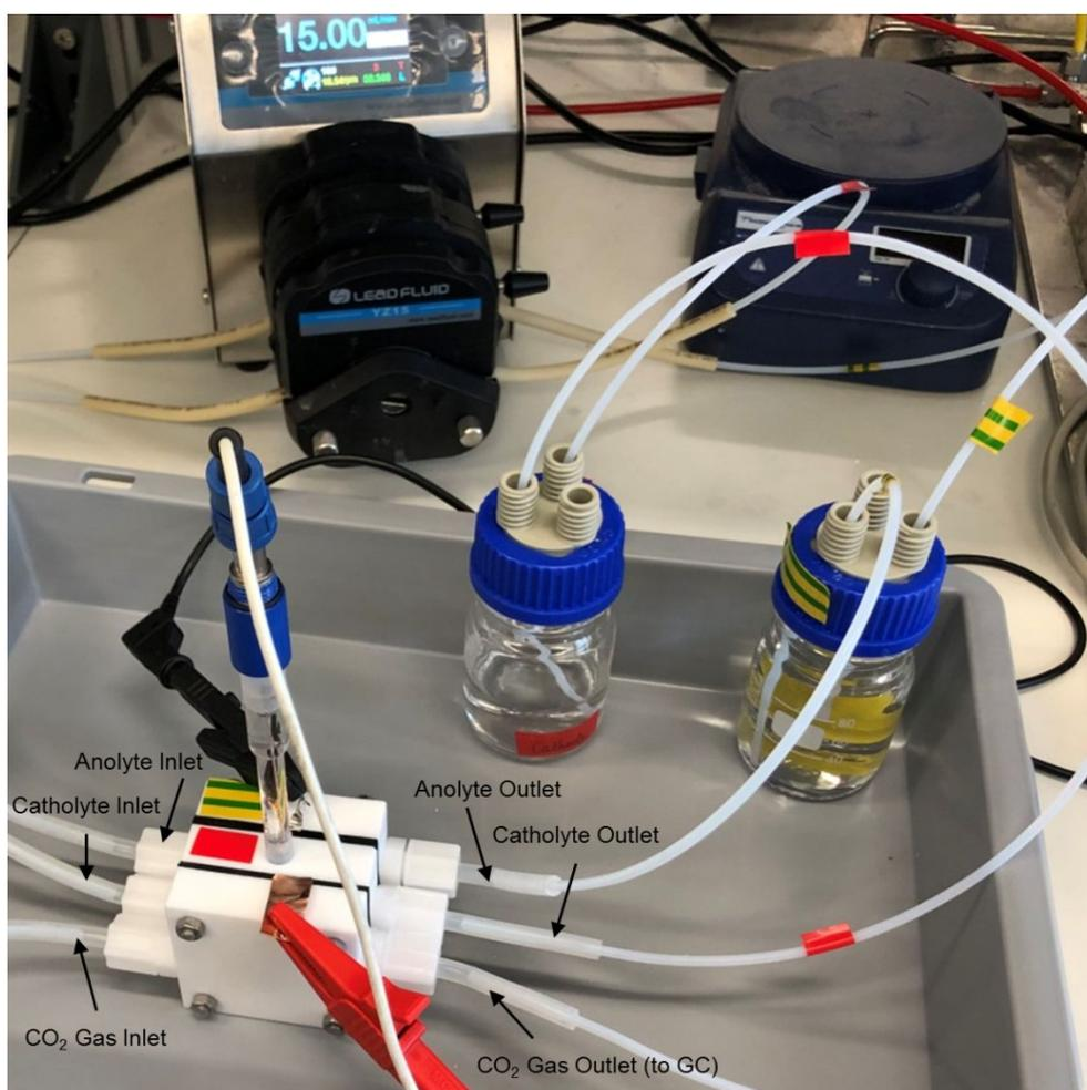
**Fig. S1:** Assembled cell and labelled inlet and outlets for the electrolyte and CO<sub>2</sub>. The catholyte and anolyte are pumped through the cell from separate reservoirs.
