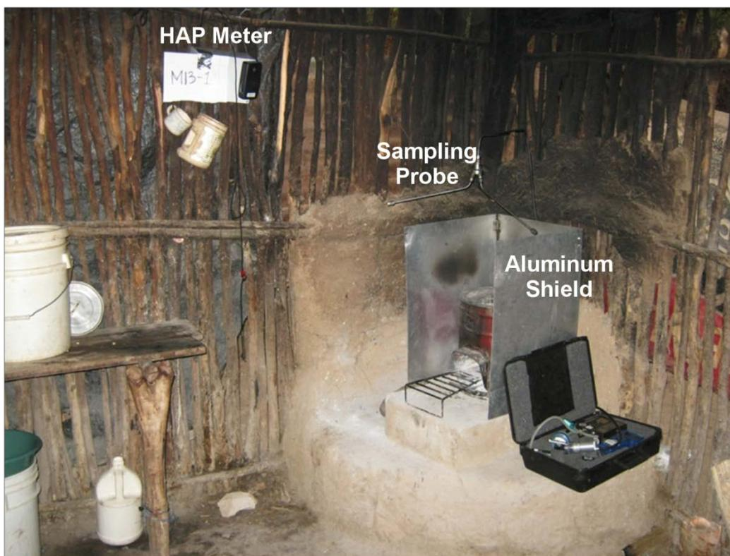
**Figure S1.** Stove emissions sampling configuration.
