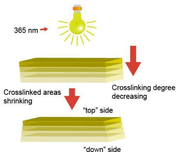
Figure S1. A sketch showing the definition of “top” side and “down” side of the photocrosslinking PVDF@PAM film.
