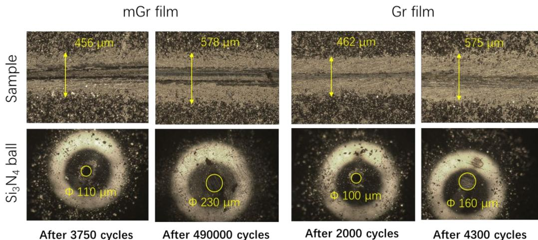
Figure S3 Optical images of the wear tracks on the mGr film, Gr film and the wear scars on their counterpart balls.
