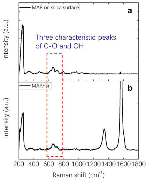
Figure S1. Raman spectrum of (a) MAP on silica surface and (b) graphene/MAP compounds.
