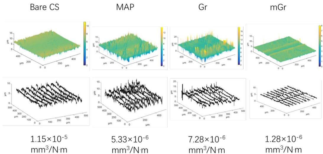
Figure S2 The 3D morphology and 2D profiles obtained from the wear track on the bare carbon steel substrate, MAP layer, Gr film, and mGr film
