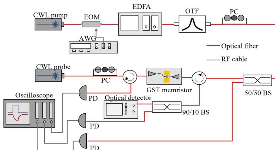
Figure S4. Experimental setup for all-optical switching. CWL: continuous-wave laser; EOM: electro-optic modulator; AWG: arbitrary waveform generator; EDFA: erbium-doped fiber amplifier; OTF: optical tunable filter; PC: polarization controller; PD: photodiode; BS: beam splitter.
