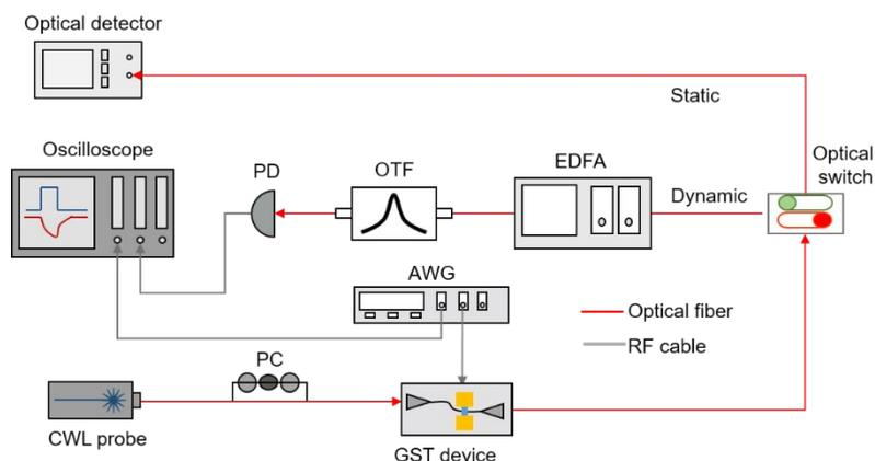
Figure S1. Experimental setup for device characterization. CWL: continuous-wave laser; PC: polarization controller; AWG: arbitrary waveform generator; EDFA: erbium-doped fiber amplifier; OTF: optical tunable filter; PD: photodiode.
