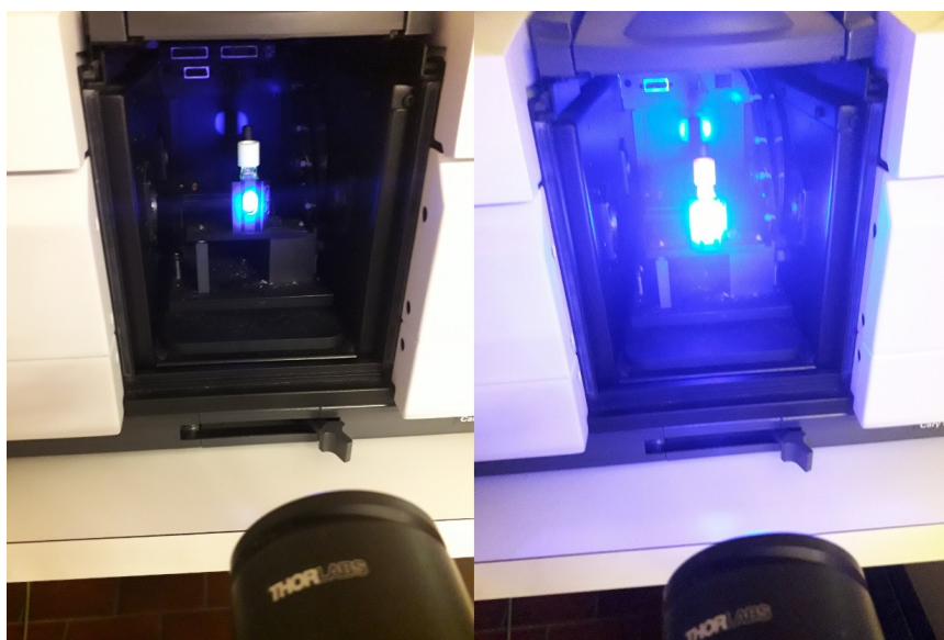
Figure S8: Setup used for photostability studies. Cuvettes with deoxygenated solutions were irradiated with a collimated 455 nm LED (M455L3-C1, Thorlabs) in the sample chamber of the Cary 5000 spectrophotometer (from Varian). The cuvette holder permits LED illumination of the whole UVVis detection volume at right angle to the detection beam. For clarity, the LED power was significantly reduced in the left part of the figure. Further details are given in the text.
