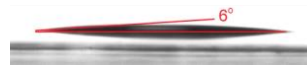
Figure S1. Contact angle test of muscovite mica and Bi(NO 3 ) 3 /(CH 2 OH) 2 .
