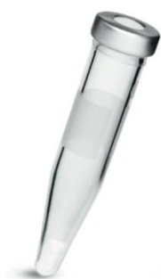
Figure S1. Reaction vial (0.5 ml – 2 ml) used for the transamidation reactions
