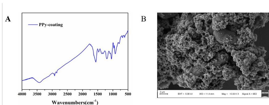
**Fig.S2** A. The FTIR spectrum of the PPy-coating. B. SEM image of the top PPy layer.
