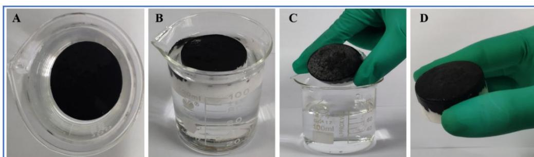
**Fig.S1** (A-B) The PPy-coated VMP foam immersed in water for 4 months. (C-D) Removed PPy-coated VMP foam from water.
