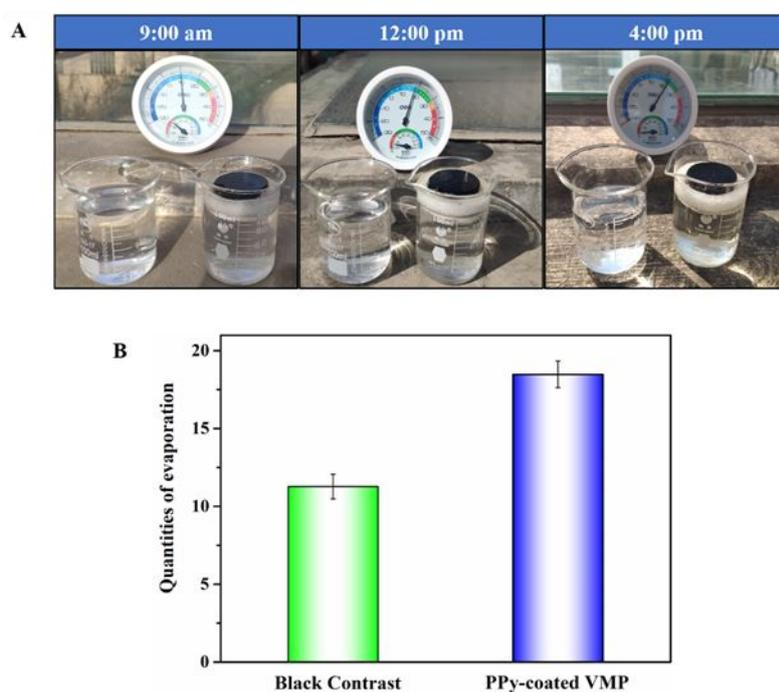
**Fig.S4** A. Photographs of the outdoor solar seawater desalination contrast experiments (from 9 am to 4 pm). B. The quantities of the simulated seawater daily evaporation under natural sunlight.
