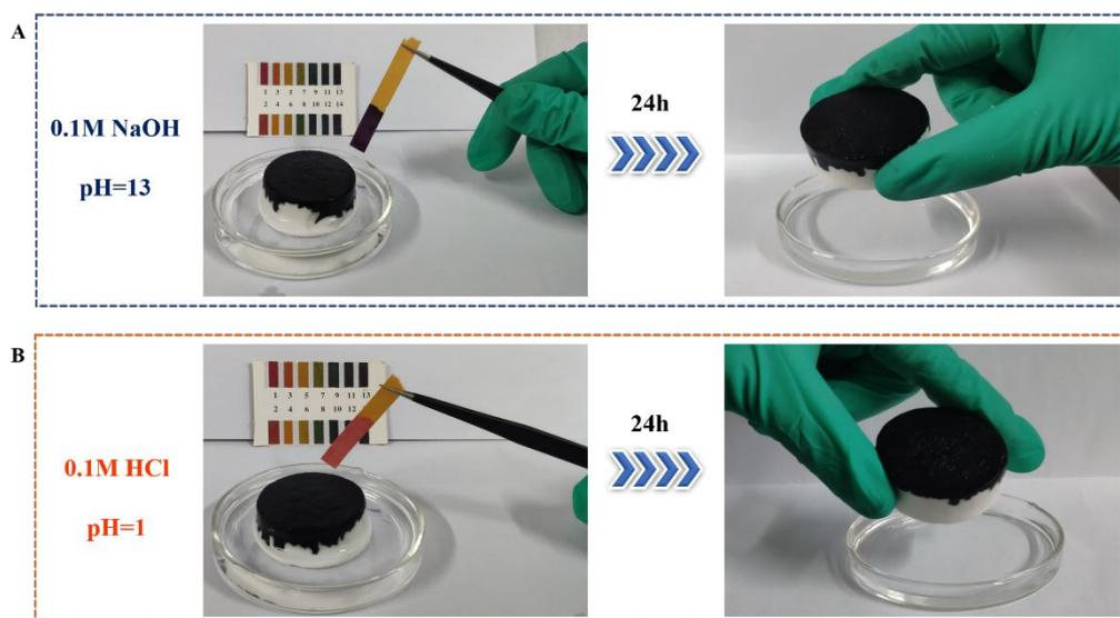
**Fig.S3** Photographs of the PPy-coated VMP foam immersed in 0.1M HCl (A) and 0.1M NaOH (B) for 24h.
