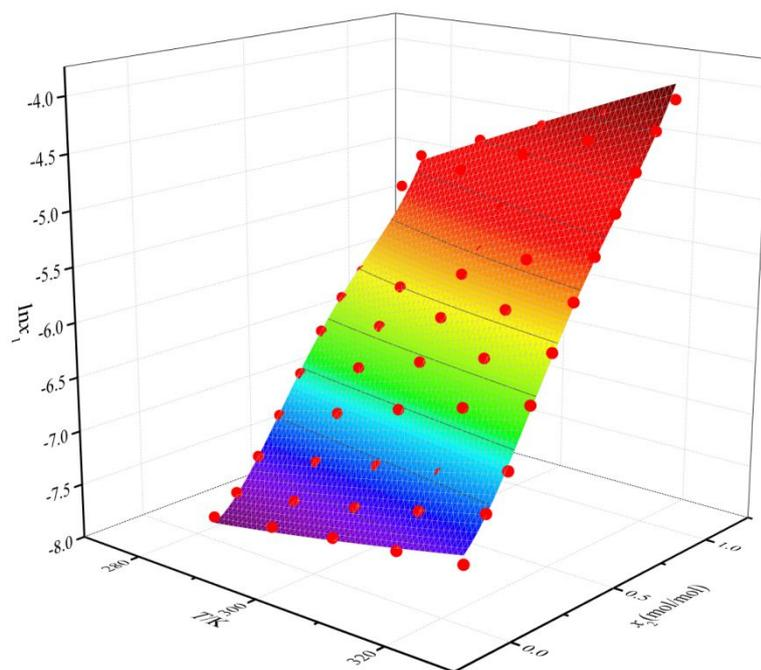
**Figure S1.** Apelblat-Jouyban-Acree model fitting plot of  $\ln(x_1)$  versus  $T$  (from 283.15 to 323.15 K) and  $x_2$  (from 0.000 to 1.000) for monosodium fumarate solubility in the full range in water + methanol.
