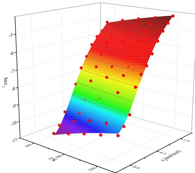
**Figure S3.** Apelblat-Jouyban-Acree model fitting plot of  $\ln(x_1)$  versus  $T$  (from 283.15 to 323.15 K) and  $x_2$  (from 0.000 to 1.000) for monosodium fumarate solubility in the full range in water + 2-propanol.
