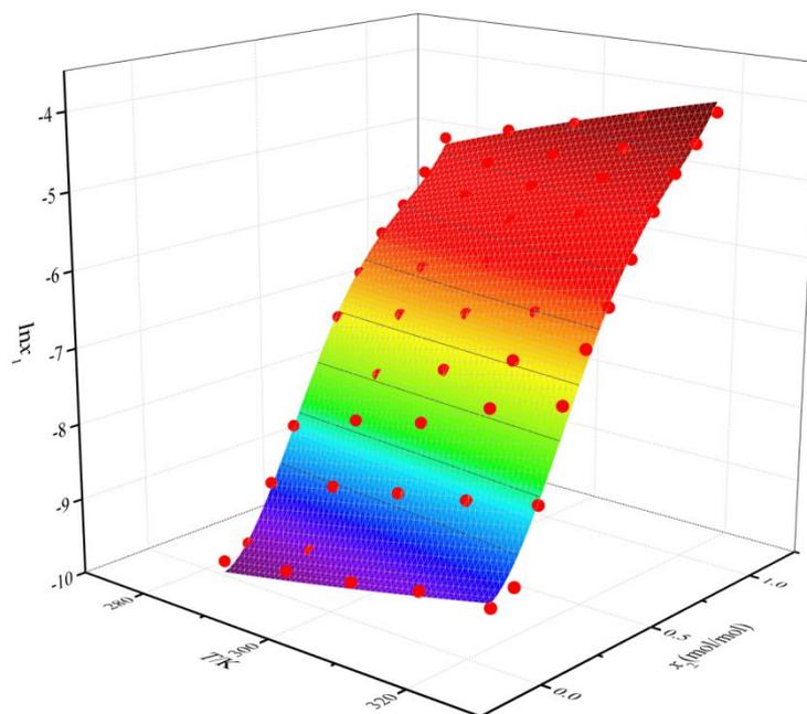
**Figure S2.** Apelblat-Jouyban-Acree model fitting plot of  $\ln(x_1)$  versus  $T$  (from 283.15 to 323.15 K) and  $x_2$  (from 0.000 to 1.000) for monosodium fumarate solubility in the full range in water + ethanol.
