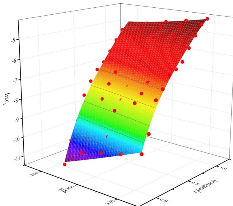
**Figure S4.** Apelblat-Jouyban-Acree model fitting plot of  $\ln(x_1)$  versus  $T$  (from 283.15 to 323.15 K) and  $x_2$  (from 0.000 to 1.000) for monosodium fumarate solubility in the full range in water + acetone.
