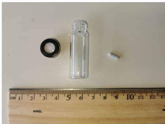
Figure S1. Screw cap fitted with a PTFE-faced silicone septum, 1-dram vial, and PTFE-coated stir-bar used in optimization studies and for isolated yields at up to 0.5 mmol scale.
