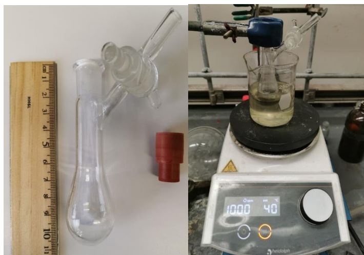
Figure S2: (Left) the Schlenk tube and rubber septum used in the benchtop reaction (Table S1, entry 21); (Right) the reaction vessel in the oil bath (Table S1, entry 21).
