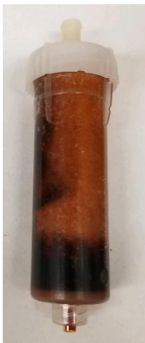
Packed bed of K_3PO_4 after use.
