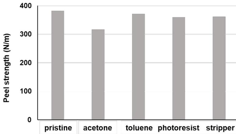
**Figure S1.** The peel strength of PSA-1 tape before and after solvent treatment. As the developing and stripping processes for photolithography need less than 1 min, the PSA-1 tape adhered to a SUS plate was immersed in the various solvents for 1 min and subject to 180° peel test. The little change in peel strength after solvent treatment means that PSA-1 tape is compatible with the photolithography process.
