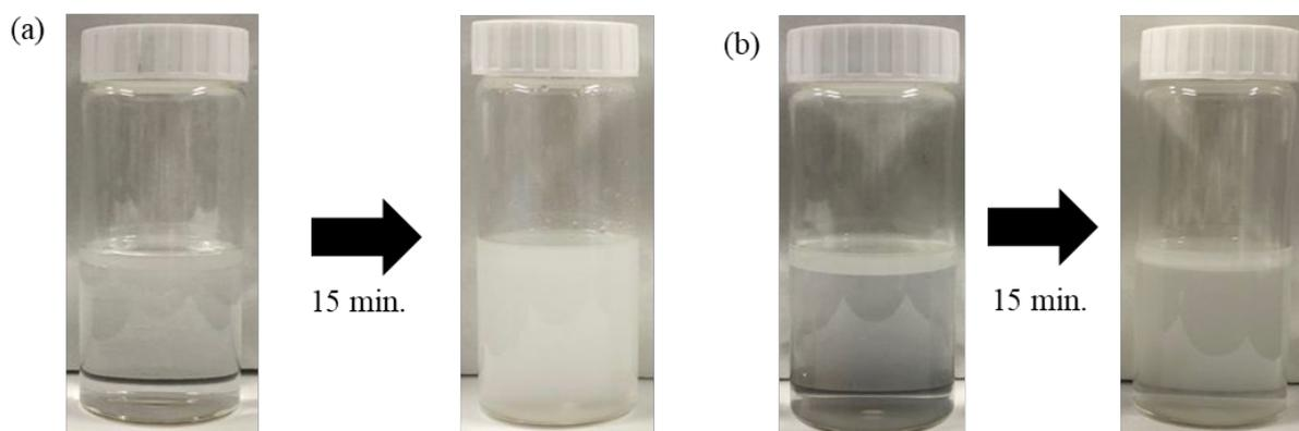
**Figure S5.** Toluene/water bilayers (a) with and (b) without oligomer MA-1 15 min after mixing.
