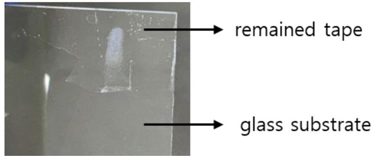
**Figure S6.** Reminders after detachment of the PSA-0 tape from a glass substrate.
