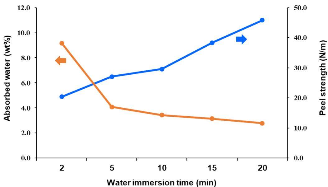
**Figure S8.** The weight percentage of the absorbed water in wr-PSA and the peel strength of wr-PSA over water immersion time at 25 °C.
