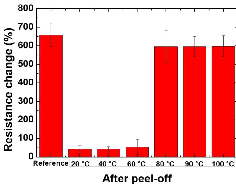
**Figure S11.** Resistance change of the water-treated AgNWs/1.4-µm-thick PET electrodes upon peeling-off after maintaining at various temperatures for 20 min. The reference refers to samples that did not experience water treatment and drying at high temperatures.
