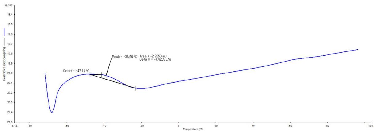
**Figure S3.** A DSC graph of polymer 1 obtained by increasing the temperature from -70 to 100 °C.
