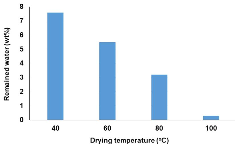
**Figure S10.** The weight percentage of the remained water in PSA-1 after drying at 40 °C, 60 °C, 80 °C and 100 °C.
