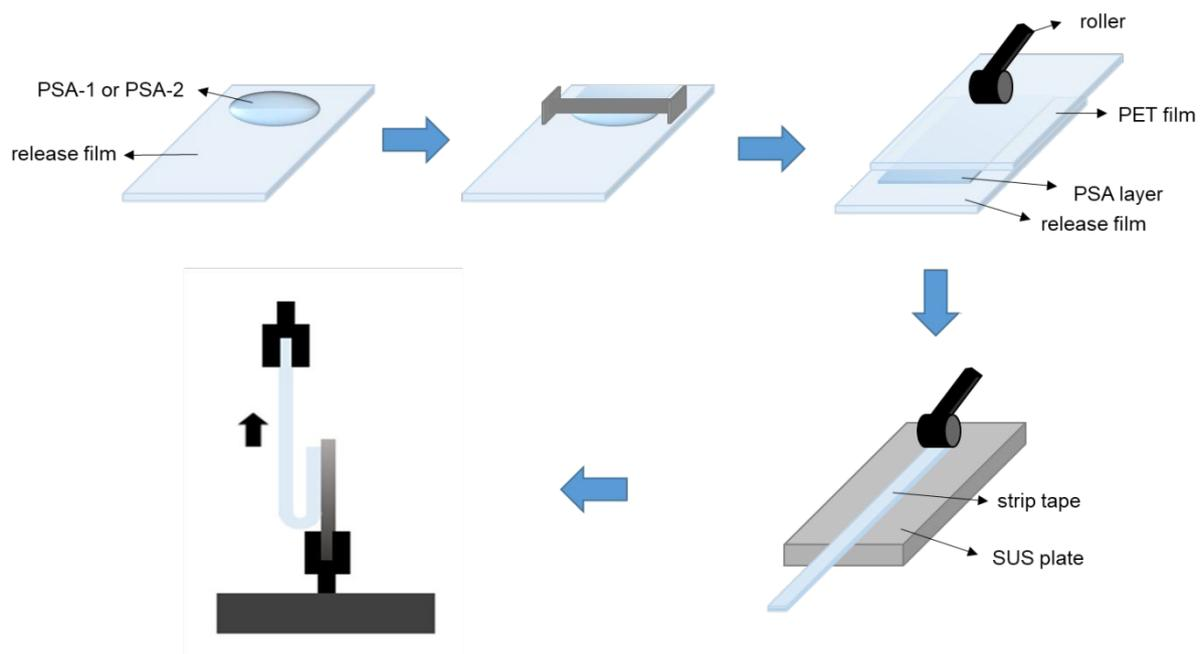
**Figure S2.** The schematic for the peel strength test.
