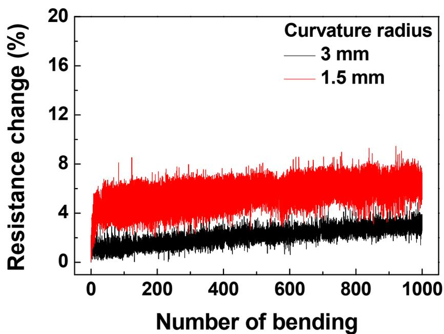
**Figure S9.** Resistance change of the AgNWs/1.4- $\mu$ m-thick PET electrode with the bending numbers employing bending radii of 1.5 and 3 mm.
