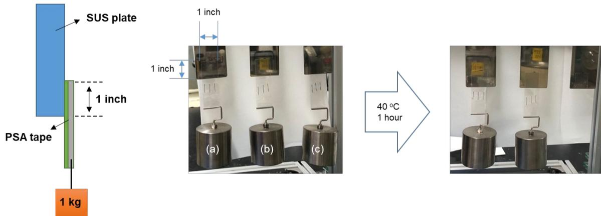
**Figure S7.** The shear resistance test of (a) PSA-0, (b) PSA-1 and (c) PSA-2 tapes. The weight with 1 kg was hung to the PSA tapes adhered to a SUS plate in a dimension of 1 inch by 1 inch, which kept in 40 °C for 1 h. While the time to shear failure for the PSA-0 and PSA-1 tapes exceeded 1 h ( $t > 1$  h), that for the PSA-2 tape was 15 min ( $t = 15$  min).
