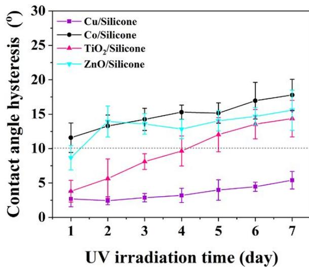
Fig. S4 Water contact angle hysteresis of the obtained monoliths as a function of UV irradiation time.
