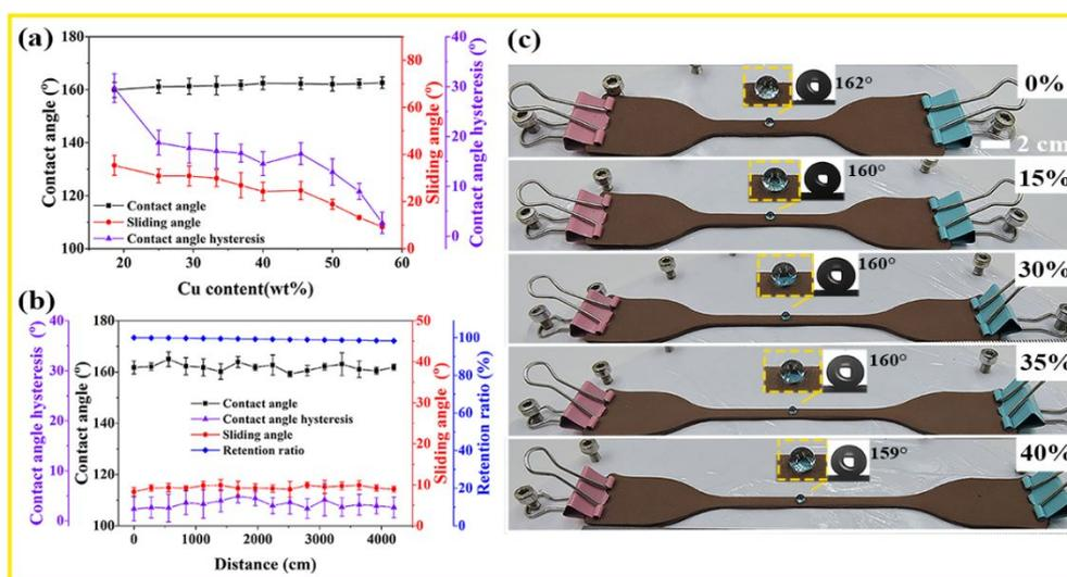
Fig. S1 (a) Relationship between contact angles, sliding angles, contact angle hysteresis and the amount of copper addition; (b) Friction and wear performance test of Cu/silicone; (c) Repellency of water after Cu/silicone is stretched to different lengths.
