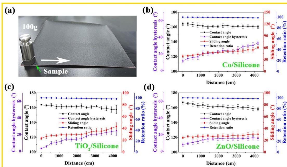
Fig. S5 Durability of the superhydrophobic monoliths. (a) Optical image. Relationship between contact angle, sliding angle, contact angle hysteresis, retention ratio and abrasion distance of Co/silicone (b), TiO<sub>2</sub>/silicone (c), ZnO/silicone (d).
