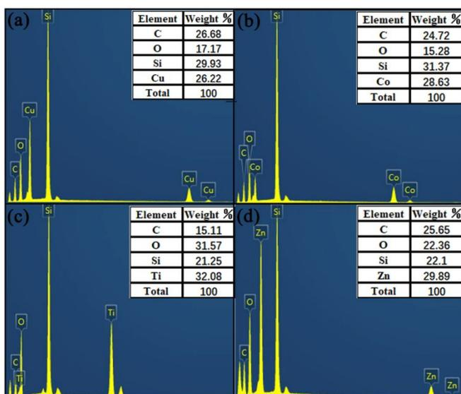
Fig. S3 EDS images and the atom percent of elements in the four types composite monoliths. (a) Cu/silicone; (b) Co/silicone; (c) TiO<sub>2</sub>/silicone; (d) ZnO/silicone.
