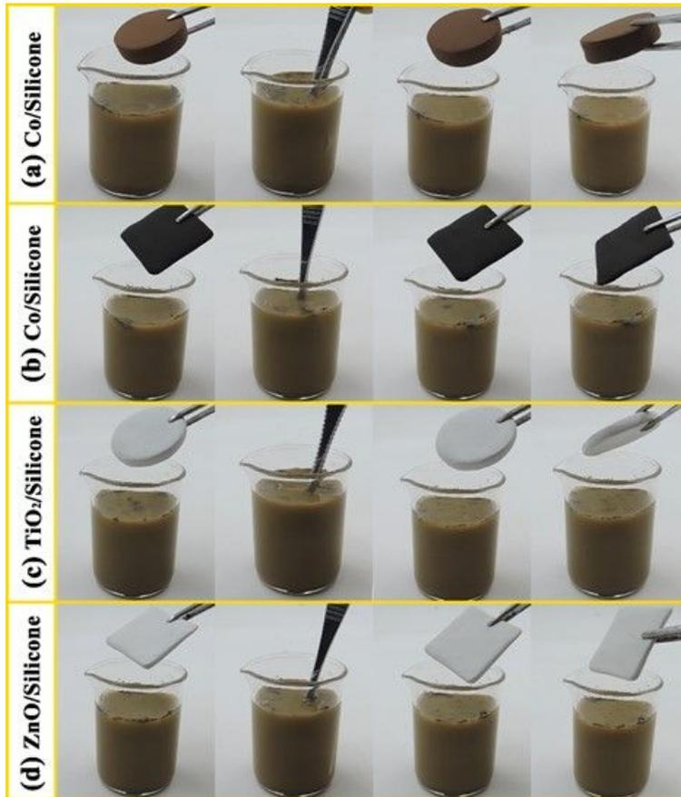
Fig. S6 Self-cleaning properties of the obtained composite monoliths.
