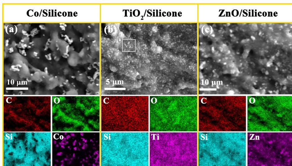
Fig. S2 SEM image and element distribution mapping of the Co/silicone, TiO<sub>2</sub>/silicone and ZnO/silicone.
