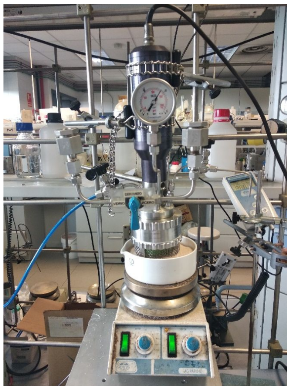
Figure S7. Reactor running a catalytic test on Reactor BüchiGlasUster™ with a sand bath.
