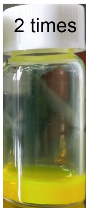
Figure S8 Photographs of CPB-2M NCs in 1-octane after two purification cycles.
