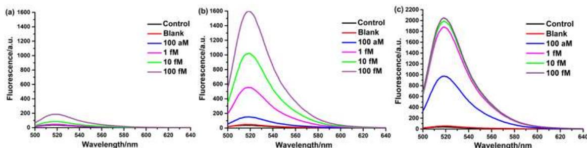
**Figure S3.** Effect of the reaction time of Cas12a cleavage on CAL-LAMP-based miRNA detection. The reaction time of the Cas12a cleavage is 10 min (a), 20 min (b), and 30 min (c), respectively.
