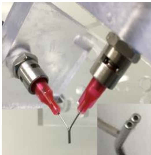
Figure S4. Image of conjugated-nozzle configuration. The inset image is enlarged view of nozzle tip.
