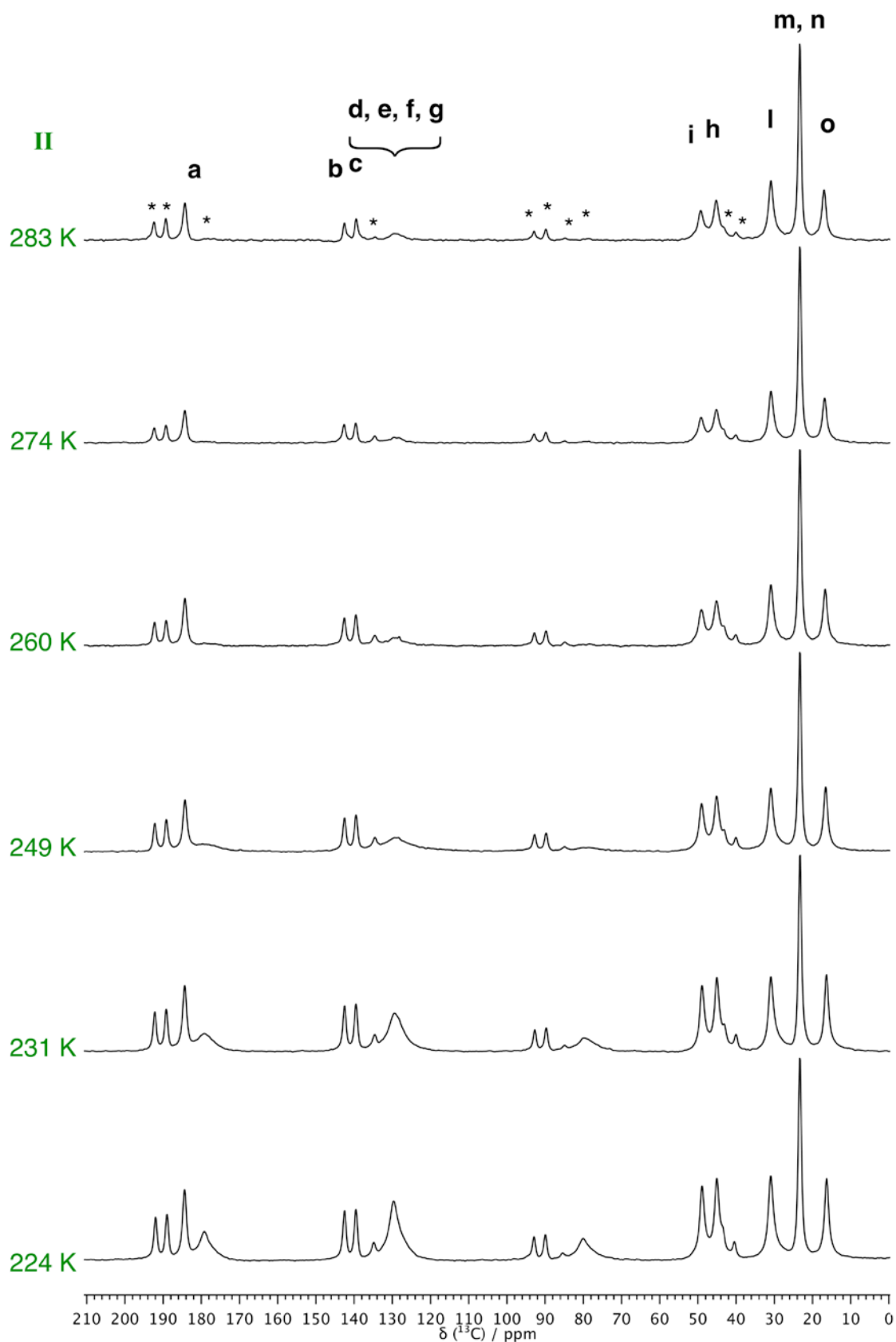
Figure 3s. ^{13}\text{C} CP-MAS spectra of IBU-S acquired in the temperature range from 283 K to 224 K (Series II). The spectra were recorded at a magnetic field of 9.4 T and magic angle spinning frequency of 5000 \pm 10 Hz. All the experimental details are reported in Table 1s. Spinning sidebands are marked with asterisks.
