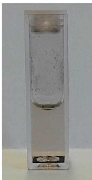
Figure S2: Redispersion behavior of lyophilized powder of BSA-coated AuNR No. 15 without additional lyoprotecting agents. The powder did not redisperse spontaneously in Milli-Q water at pH 12.
