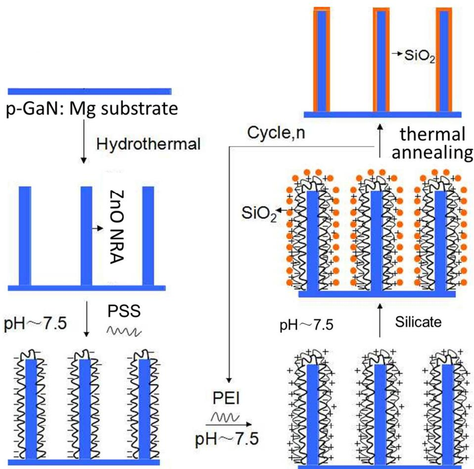
**Figure S1.** Schematic flow charts for the preparation of ZnO/SiO<sub>2</sub> core/shell NRAs.
