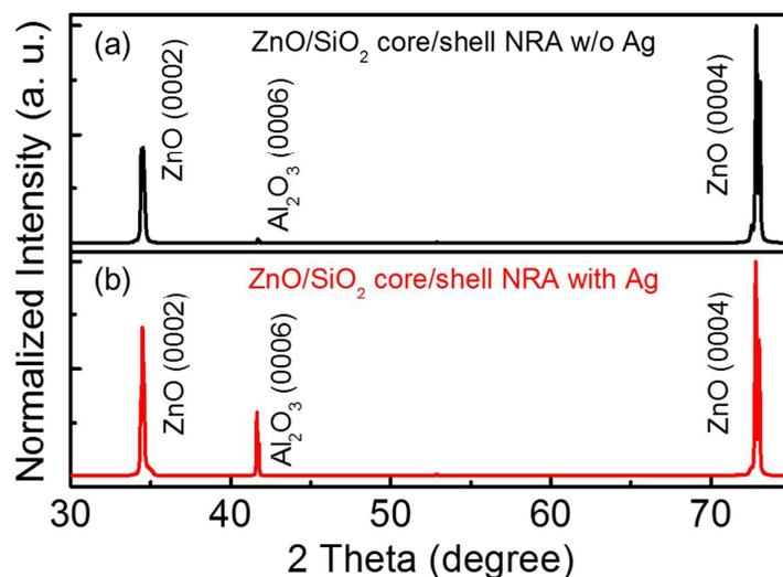
**Figure S2.** XRD patterns of the ZnO/SiO<sub>2</sub> core/shell NRAs without (a) and with (b) Ag NPs decoration, respectively; the thickness of SiO<sub>2</sub> shell is 12 nm.
