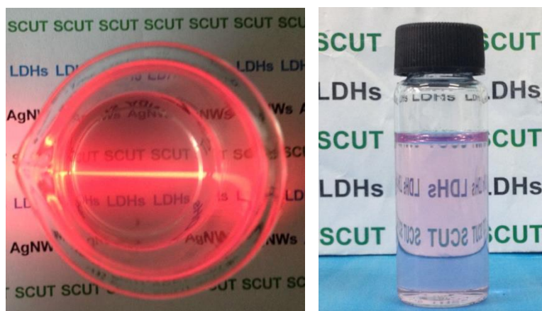
Fig.S6 Obvious Tyndall effect is observed for Co-Al LDH nanosheets colloidal suspension, which has an outstanding stability of more than 6 months without any sediment.
