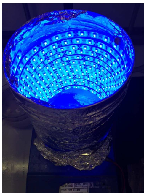
Figure S2: Visible light photoreactor used in this study which was constructed from a commercial LED strip light wound around the inside of a beaker.
