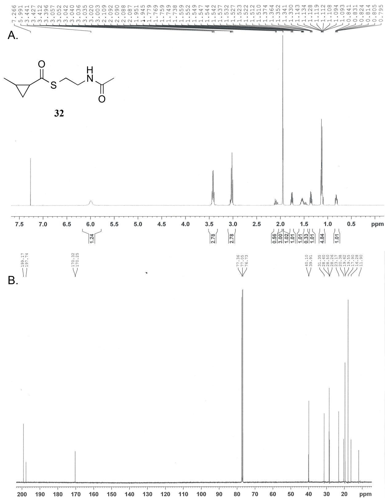
Figure S52. NMR spectra of S -(2-acetamidoethyl) 2-methylcyclopropane-1-carbothioate ( 32 ) A) 1 H NMR spectrum B) 13 C NMR spectrum
