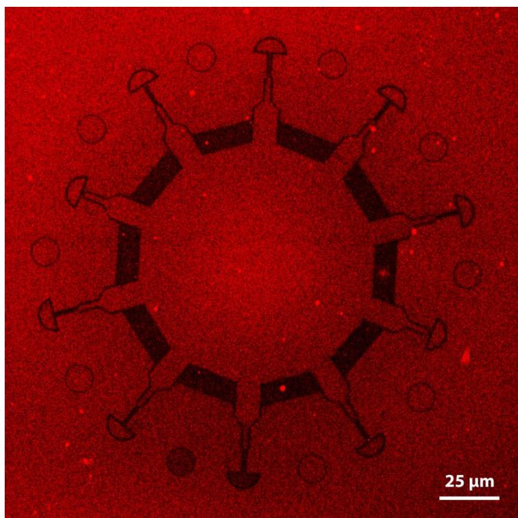
**Figure S8:** Fluorescence micrograph showing the surface coverage of an e-beam patterned Teflon AF surface by bulk exposure to a suspension of single unilamellar nanovesicles. The red colored areas are unexposed Teflon AF, covered with a lipid monolayer resulting from adhesion, rupture and fusion of SUVs, the dark areas are the lipophobic e-beam exposed structures.
