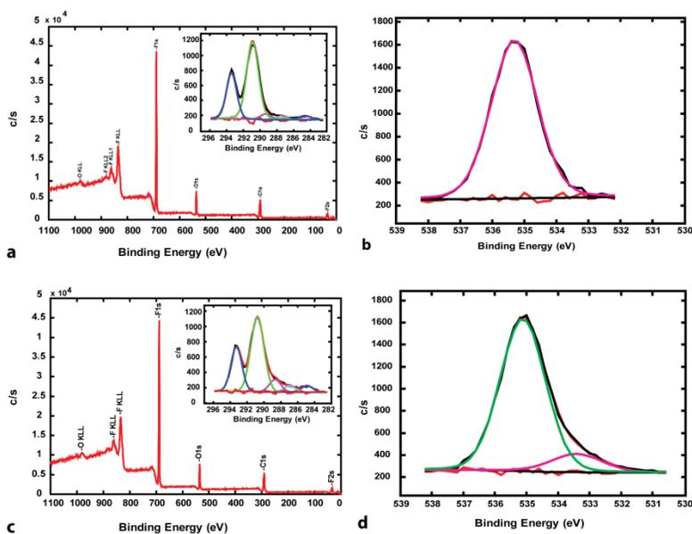
**Figure S2:** a) Carbon XPS spectra of unmodified Teflon AF. b) Oxygen XPS analysis of unmodified Teflon AF. c) Carbon XPS spectra of e-beam irradiated Teflon AF. d) Oxygen XPS analysis of e-beam irradiated Teflon AF.
