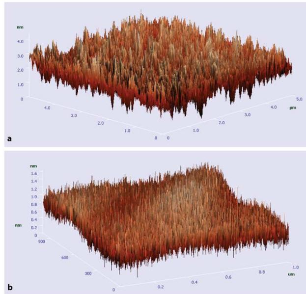
**Figure S4:** AFM images of Teflon AF surfaces roughness before and after exposure to e-beam radiation, **a)** Unexposed Teflon AF, **b)** Exposed Teflon AF. The exposed area has a 3x reduced surface roughness.
