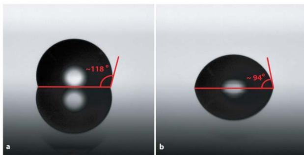
**Figure S1:** Water contact angles on **a)** Teflon AF, **b)** on e-beam exposed Teflon AF
