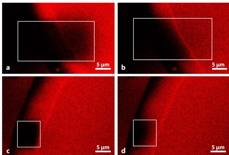
**Figure S5:** Confocal images of two exemplary FRAP experiments. **a-b)** demonstrating faster recovery on unbleached Teflon vs exposed edge, where time between (a) and (b) is 3 minutes. **c-d)** showing different recovery rate in radial vs. axial direction, where time between (c) and (d) is 6 minutes.
