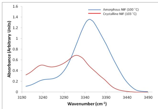
Supporting Figure 3. FTIR spectra revealing an amorphous to crystalline transition of NIF from 100 °C (amorphous form) to 103 °C (crystalline form).
