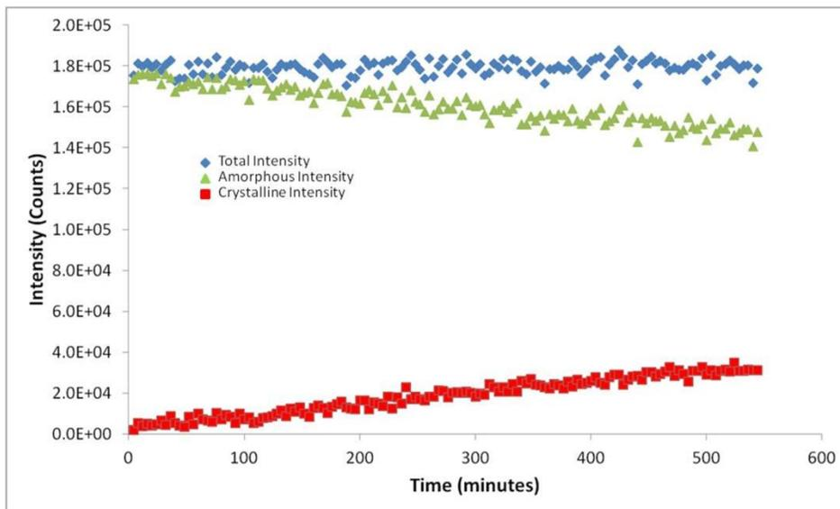
Supporting Figure 1. A representative plot of the total (crystalline + amorphous), amorphous and crystalline integrated intensity during the isothermal crystallization studies of amorphous NIF-PVP (10% w/w) at 70°C. Initially, the sample was X-ray amorphous (no evidence of crystallinity), and at the end of the experiment, it was ~15% crystalline. This data indicates that the % crystallinity can be expressed as crystallinity index.<sup>1</sup>
