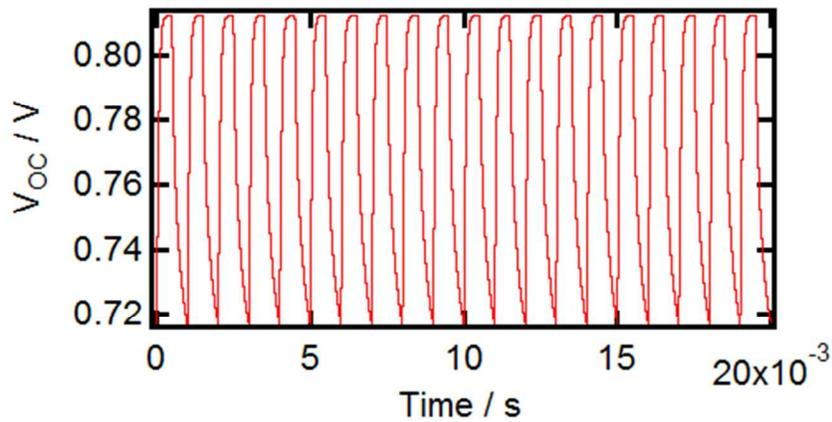
**Figure S4.** Simulated  $V_{OC}$  as a function of time under LED modulating frequency of 1000 Hz and an equivalent white light background excitation intensity of  $1 \text{ mW/cm}^2$  and a modulated LED peak intensity of  $25 \text{ mW/cm}^2$ .
