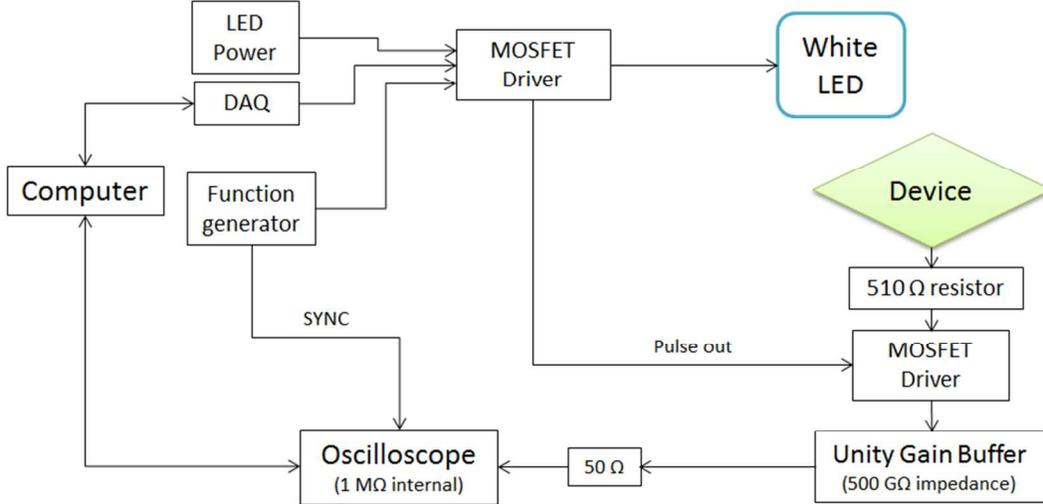
Figure S2. CE measurement setup.<sup>1</sup>
