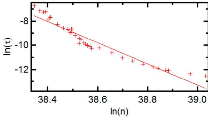
**Figure S6.** Natural log of the small perturbation carrier lifetime,  $\tau$ , plotted as a function of  $V_{oc}$ .
