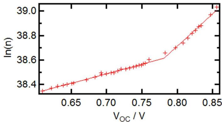
**Figure S8.** Natural log of carrier density plotted against  $V_{oc}$ , the raw data were fitted with by two exponentials to yield more accurate extrapolation of  $V_{oc}$ .
