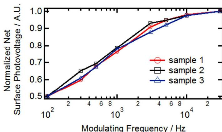
**Figure S9.** Intensity-modulated SKPM with probing intensity of 12.5 mW/cm<sup>2</sup> and no background illumination measured on three different samples prepared identically.
