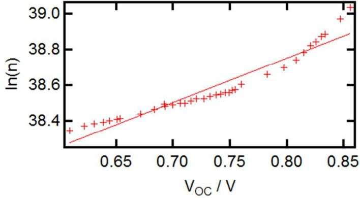
**Figure S7.** Carrier density,  $n$ , plotted as a function of  $V_{oc}$ . The solid line is a fit to  $n = n_0 \exp(\gamma V_{oc})$ .<sup>4</sup> Here,  $n$  is the carrier density measured from charge extraction, corrected for recombination during extraction and device geometric capacitance.  $n_0$  and  $\gamma$  are fitting parameters. The corrected  $n$  vs.  $V_{oc}$  data show the largest deviation from the single exponential form.
