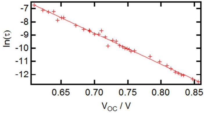
**Figure S5.** Natural log of the small perturbation carrier lifetime,  $\tau$ , plotted as a function of  $V_{oc}$ .
