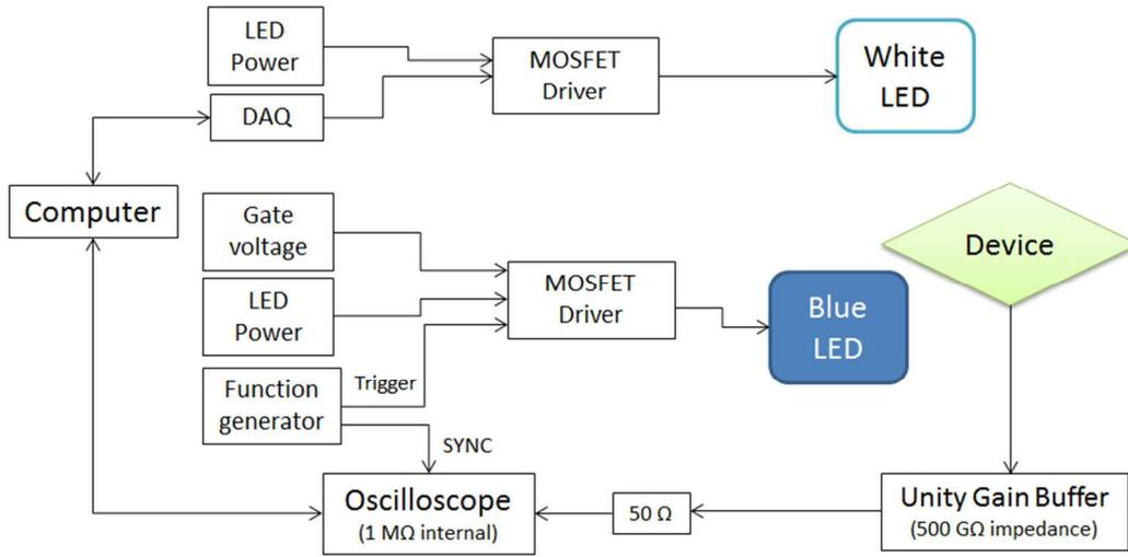
Figure S1. TPV measurement setup as used previously.<sup>1</sup>
