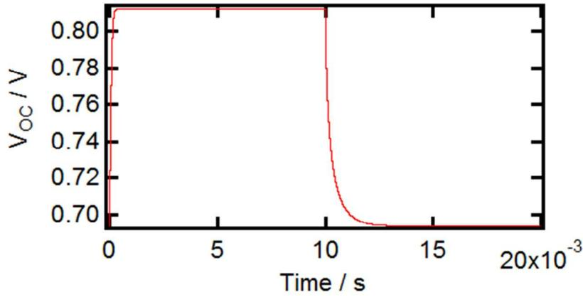
**Figure S3.** Simulated  $V_{OC}$  as a function of time under LED modulating frequency of 50 Hz and an equivalent white light background excitation intensity of  $1 \text{ mW/cm}^2$  and a modulated LED peak intensity of  $25 \text{ mW/cm}^2$ .
